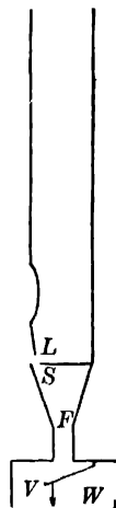
Fig. 47. A flue organ-pipe. Air escaping through the slit S impinges on the lip L and produces an edge tone, thus setting the column of air inside the pipe into vibration.
